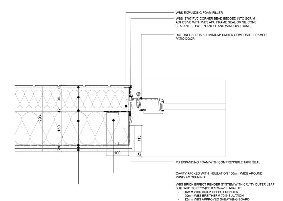
150mm LIGHT STEEL FRAME SYSTEM WITH 150mm MINERAL
